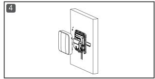
Secure the casing by tightening the security screw. Peel off and discard the protective plastic film covering.
